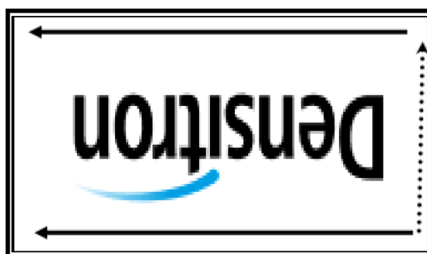
Fig. 2 Reverse scan (Pin 4, LR/UD = Low)
