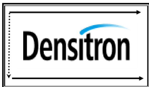
Fig. 1 Normal scan (Pin 4, LR/UD = High or NC)
